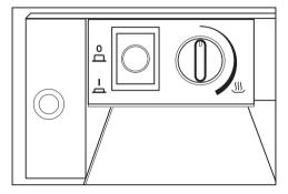
The controls include the temperature selector and the On/Off button. They are only visible when the drawer is open.
